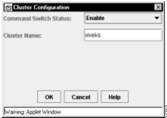
Figure 4-2 Enable Command Switch
