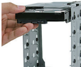
6.3 Slide the HDD into the drive bay
