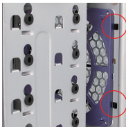
8.1 Push the hooks marked in red circles.
