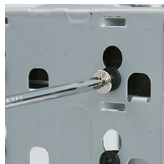
6.4 Screw up and fasten HDD on the cage *Handle with care because HDD is likely to be damaged by careless management
