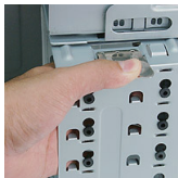
6.2 Push the handle down and pull the large cage out
