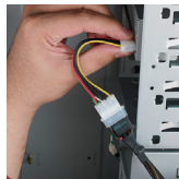
11.3 The 4 pin female connector can still used for another device.
