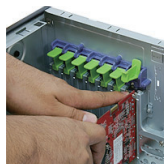
7.2 Insert your add on card into the right slot
