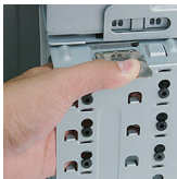
6.5 Slide the large cage into drive bay and fasten the thumb screws
