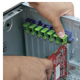
7.3 Push down the kit to fasten the add on card
