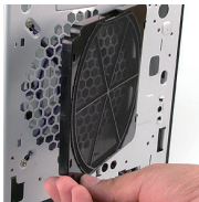
8.2 Detach the air filter to clean.
