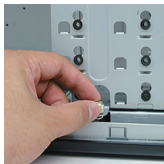
6.1 Take off the thumb screw on the large cage
