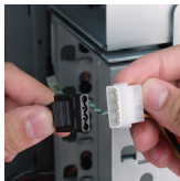
11.2 Connect the 4 pin male connector to a peripheral 4 pin connector from power supply.
