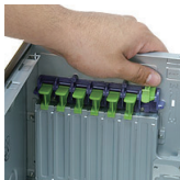
7.1 Loosen the kit above the slot you want to install your add on card in and remove the metal cover by your flat screwdriver.
