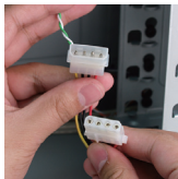
11.1 Find the front panel LED cable. (1x 4 pin male connector & 1x 4 pin female connector)
