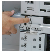
5.4 Slide the small cage into drive bay, make sure the cage is properly positioned
