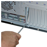
7.1 Loosen the kit above the slot you want to install your add on card in and remove the metal cover by your flat screwdriver.
