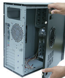
1.3 Roll the side cover anticlockwise to open
