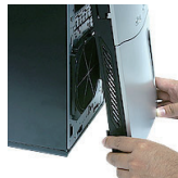
1.4 Press the 2 buttons on both sides of lower front panel and carefully pull down and forward to move the front panel
