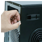
1.1 Take off the thumb screws on the back panel
