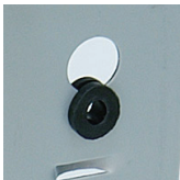
HDD cage with Shockproof Rubber Pads
