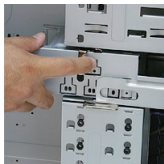
5.1 Pull the handle and cage backwards to take off the small cage
