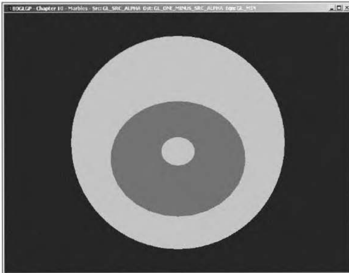
Figure 5.10 Disks drawn with GL_MIN.
