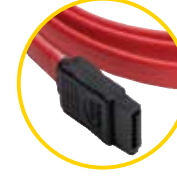
Discrete SATA (Standard, point-to-point SATA cable)
