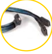
M8 to SFF-8087 (Multi-lane internal "Y" cable)
