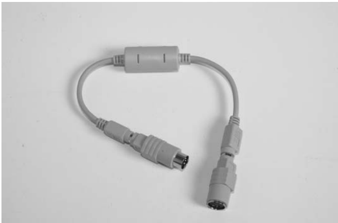
Figure 4.2 Keyghost keystroke-capturing device with some adaptors.
