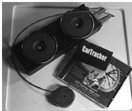
Figure 14.1 Commercially available covert vehicle tracker using GPS.
