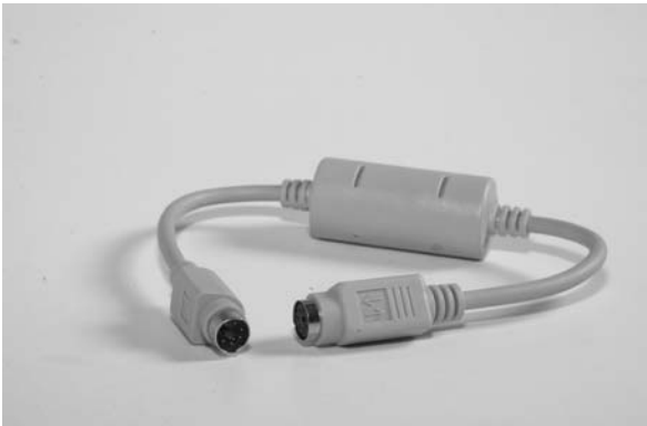
Figure 4.3 Keyghost keystroke-capturing device without adaptors.
