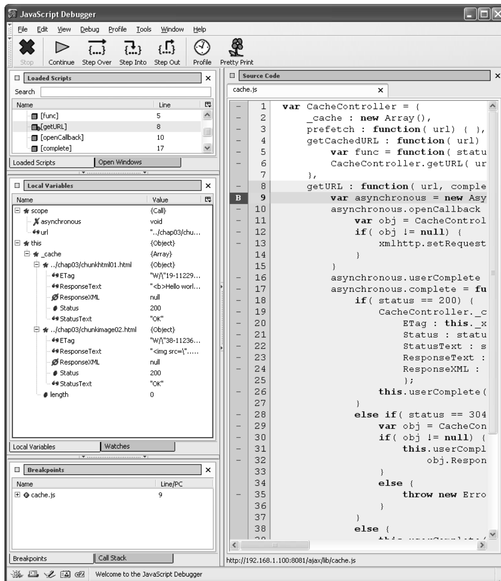
Figure 4-4. Mozilla debugger illustrating that there are two items in the cache
