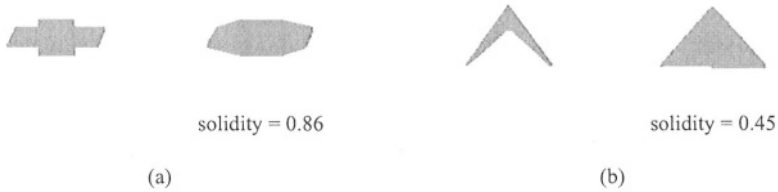
Figure 19.3. Examples of object solidities. The solidity can be computed as the area of the object divided by the area of its convex hull. (a) Solid object. (b) Less-solid object.
