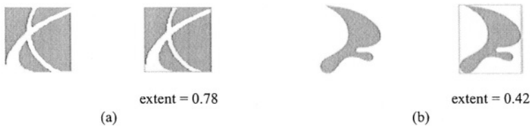
Figure 19.5. Examples of object extents. The extent can be computed as the area of the object divided by the area of its minimum bounding rectangle (MBR). (a) Object with high extent value. (b) Object with smaller extent value.
